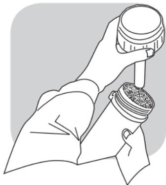
Over time the pre-filter disc will become worn. It should be replaced if it becomes torn. In any event it should be replaced every 6-12 months dependent on use.
