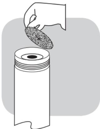
When the pre-filter disc has collected muck, dirt, sand and other debris these should be washed free from the pre-filter disc before re-inserting.
